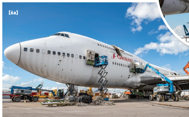
[6a] The interior of the Boeing 747 being removed. 波音747型客機內部正被拆卸。
