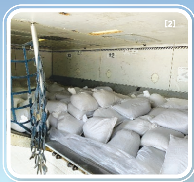
[2] Airlines add bulk such as sandbags to the cargo hold when a typhoon is approaching. 當颱風逼近，航空公司會在飛機貨艙放置沙包等壓載物。
